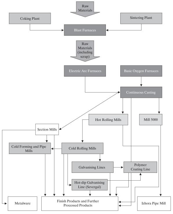
The Russian Steel Division continuously seeks to improve the efficiency of the steel production process through the implementation of its asset modernisation programme and the decommissioning of the open-hearth furnaces, the ingot casting lines and cogging facilities.
